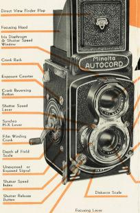
Iris Lever Direct Viewer Diaphragm Opening Index Back Cover Opening Knob 2 a 10 a Flash Synchro Contact Socket Film Loading Spool Knob Film Start Mark Taking Lens Take - un Spool Knob
